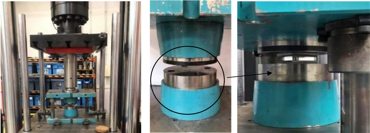
Figure 8. Instron SATEC hydraulic testing machine and setup used in joining tests.
