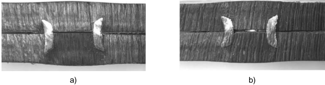
Figure 13. Cross-section of two different double-sided self-pierce riveted joints obtained ( h_0 = 8 \text{ mm} and \alpha = 45^\circ ) with a) sharp chamfered ends r_f \cong 0 \text{ mm} ; b) blunt chamfered ends r_f \cong 0.2 \text{ mm} .
