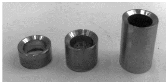
Figure 5. Manufactured rivets with different chamfered angles and initial heights
